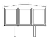
1675mm x 850mm aluminium board - curved or flat top  $3 \times A2$  poster cases  $2 \times 76$ mm diameter aluminium posts  $\pounds 1075.00 + vat$
