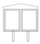
1500mm x 1200mm aluminium board - curved or flat top  $2 \times A1 \ poster \ cases$   $2 \times 76mm \ diameter \ aluminium \ posts$   $\pounds 1100.00 \ + \ vat$
